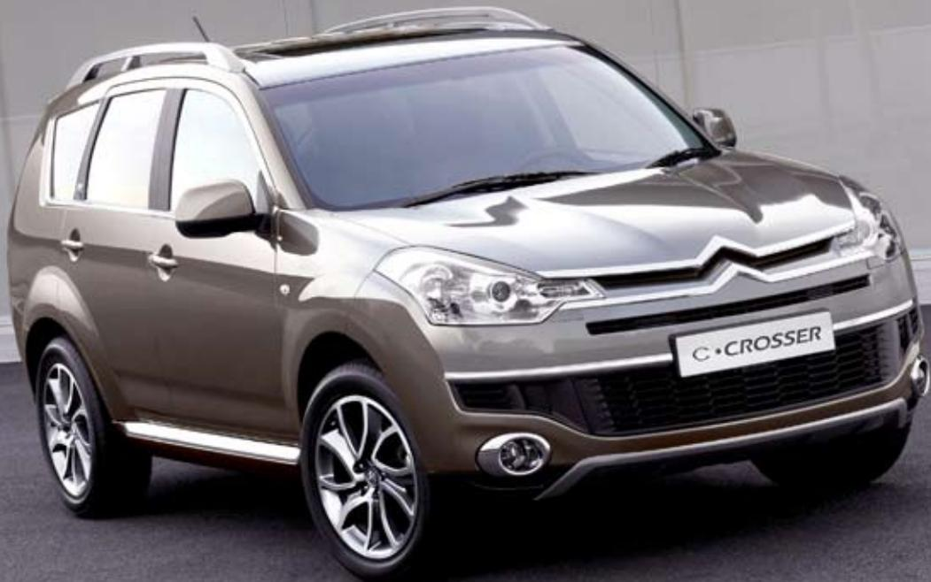
With the C-Crosser's integral transmission, drivers have a choice of three settings, dependent on road conditions and driving style: two-wheel drive, four-wheel drive and a lock setting designed for low-grip conditions. Ensuring an optimum blend of comfort, road holding and off-road capability, Citroën's new SUV is equipped with MacPherson strut front and multi-link rear suspension, combined with 18-inch Michelin tyres for added grip.
